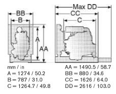
**Gen Pac** - Gen Set Engine mounted on an expandable base frame. Complete unit with engine, radiator, radiator core guard, fan, fan and belt guard providing reduced delivery time and inatallation cost and simplified transportation.
